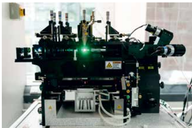
Figure 1: The high-end cell sorter (BD Influx), which allows the isolation of large and fragile cells, such as stroma cells or stem cells, the isolation of extremely small cell components, and for polarisation measurements.
