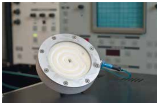
Figure 2: A newly developed module equipped with UV-C LEDs being currently tested for the continuous decontamination of the sheath fluid of cell sorters. The prototype has been developed in collaboration with the Ferdinand Braun Institute and the TU Berlin and is suitable for all currently commercially available sorters and thus could reduce the danger of contamination during the sorting process.
